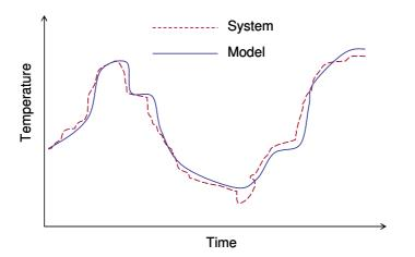
To identify a black box system a random signal (called pseudo Random Signal or PRS) input is used. This input excites the system. From the measurements of the input and output signal the system parameters can be identified and the system model can be built.
