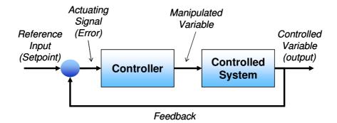
Basic elements of a feedback control system
