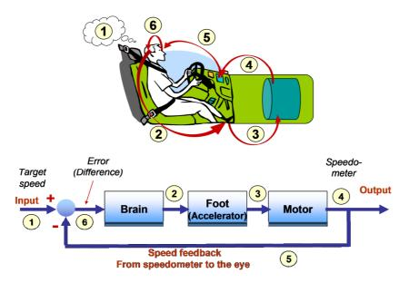
The main performance measure for a control system relates to rate of error reduction. Usually, performance is quoted in terms of the highest frequency that the control system can follow, when required to do so. All control loops tend to become unstable as higher and higher performance is sought.
